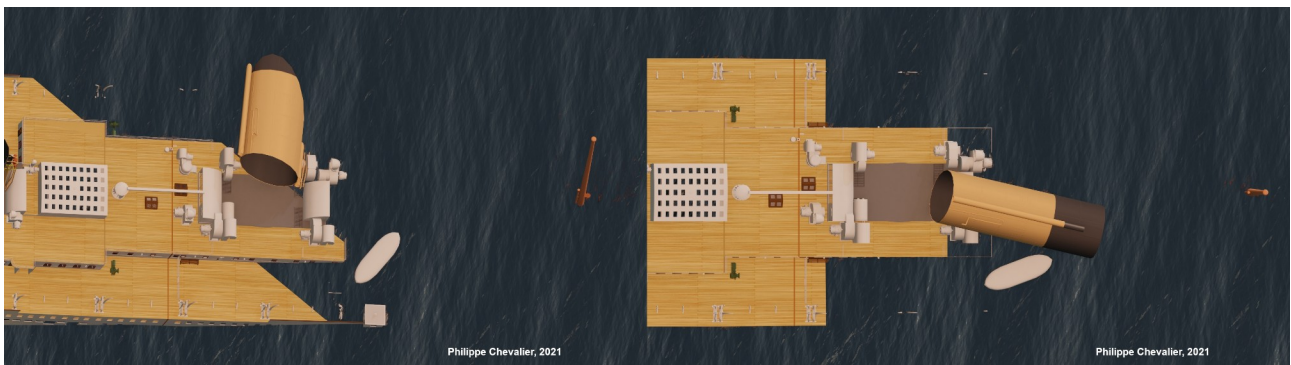
Figure 1: This reconstruction illustrates the problem of raft B being propelled aft and to starboard, if the first funnel fell to port. In contrast, the position of raft B aft and to starboard, close to Jack Thayer, is explained if the first funnel fell on the port side forward.
