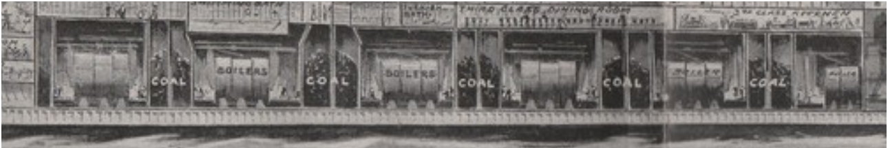
Figure 5: Representation of the six boiler rooms of the Titanic . On the left, the most forward boiler room, boiler room n° 6. It is followed by the boiler room n° 5, and so on until the boiler room n° 1.
